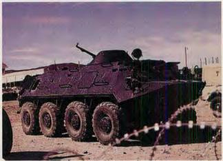
ABOVE: Amphibious, wheeled Russian APC designated BTR-60PB brandishes coaxial-mount 7.62mm PKT and heavy 14.5 KPV machine guns. LEFT: Tanker sleeps on Russian T-72, latest Warsaw Pact main battle tank. LOWER LEFT: APC crewman checks and performs light maintenance on M113 after tank "battle." LOWER RIGHT: Between battles "Red" tank crewmen pose next to T-72. Wearing replica Russian tanker berets, crewmen perform routine field maintenance.
